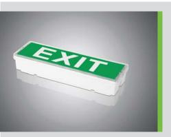
Indoor and outdoor use Polycarbonate case and glass Moisture-proof SMD LED application High energy saving Long life-time (50.000 hours) Emergency lighting function by interruption of the unswitched phase Emergency lighting function in case of low-voltage 3 hours duration in case of emergency Charge status display with green LED Test switch High-temperature Ni-Cd battery cells Overcharge and deep discharge protection Wall mounted Optional - 110 VAC compatibility
