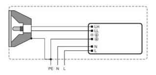
342165\_Setup for ECG Installation
